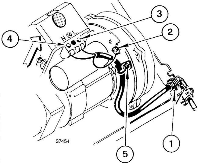
The diagram shows a burner assembly with a control box. Five numbered callouts point to specific components: 1) A wire access hole on the side of the burner housing. 2) An earth ground terminal on the control box. 3) A hot conductor terminal on the control box. 4) A neutral conductor terminal on the control box. 5) A strain relief clamp on the burner housing. The control box has terminals labeled 'N' and 'L'. A terminal with a circled 'X' is also visible. The diagram is labeled 'S7454'.
