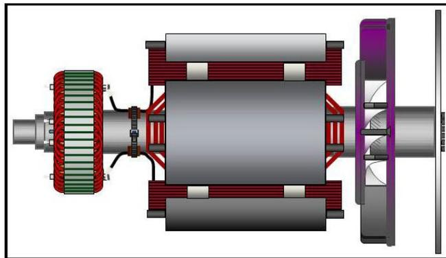
**FIGURE 20. SINGLE BEARING ALTERNATOR ROTOR SHOWING COUPLING DISCS BOLTED TO DRIVE END COUPLING HUB (AT RIGHT)**
