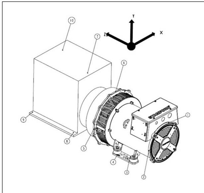
FIGURE 17. VIBRATION MEASUREMENT POSITIONS
