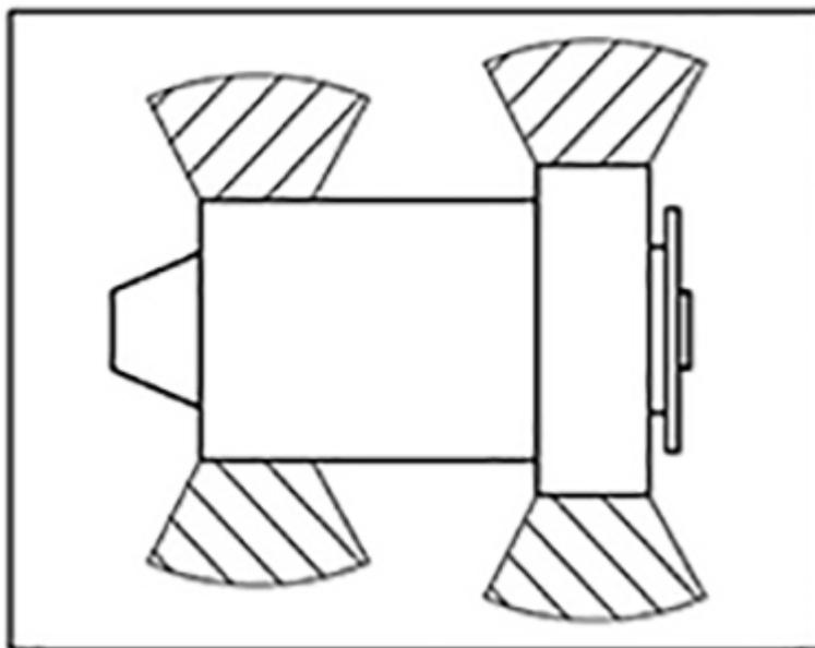
**FIGURE 5. S0/S1 ALTERNATOR HAZARD ZONES**
